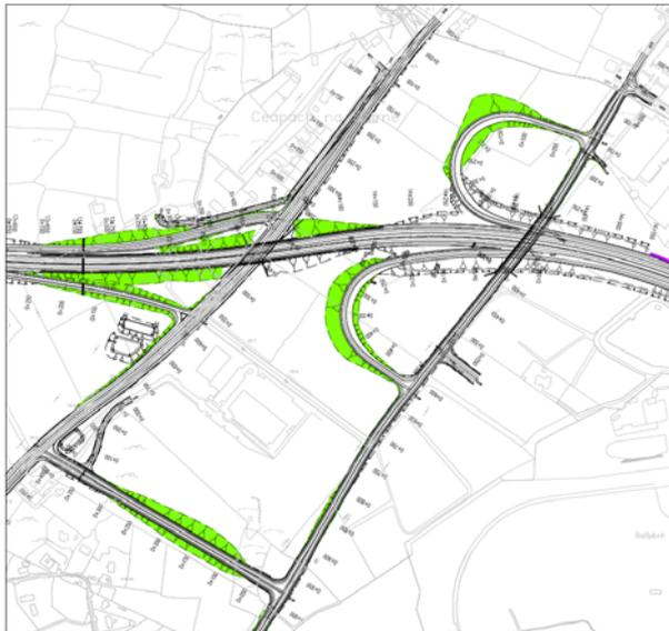
The refined N17 junction comprises a grade separated junction and associated link roads. The slip termini, as well as all junctions integral to the operation of the junction, are signalised. This junction form and modus operandi is the most suitable at this location for the following reasons:
